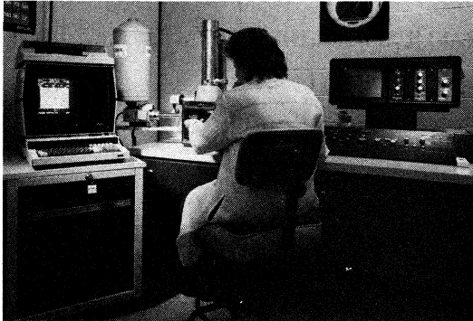
State-of-the-art SEM (Scanning Electron Microscope) and semi-quantitative EDAX (Energy Dispersive Analysis of X-rays) system with EBIC (Electron Beam Induced Current) capabilities .
